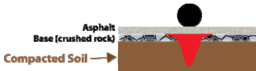
Figure 4: Stress distribution of flexible pavement [2]
